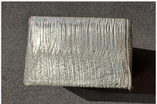
30mm thick A36 metal cut with LASER using Oxygen.
