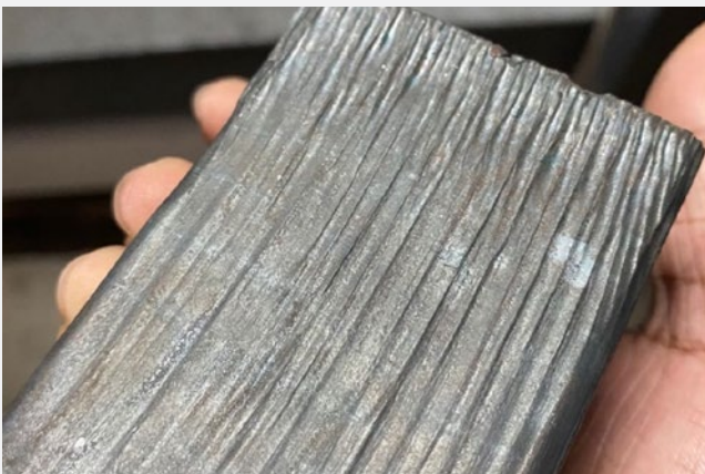
80mm thick A36 metal cut with LASER using Oxygen.
