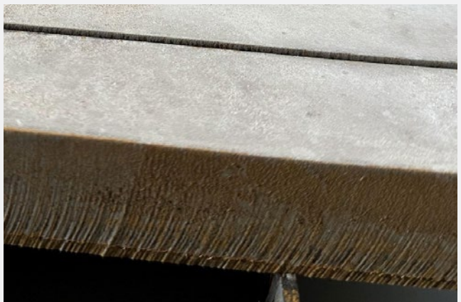
HARDOX 450 – 40mm HARDOZ material cut with waterjet machine. This photo clearly shows that no burns occur during the cutting process.
