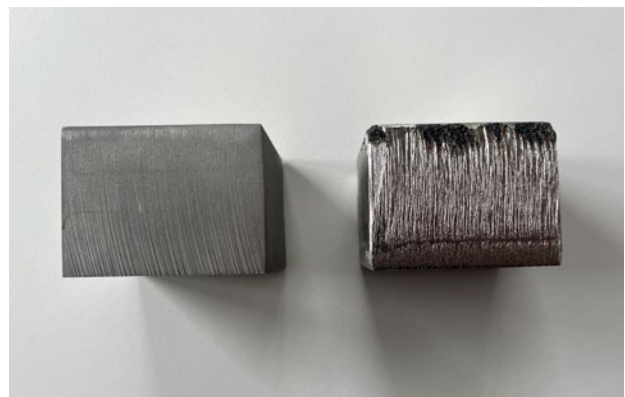
Side-by-side comparison showing the finish of the same metal part cut from a waterjet and laser cutter.
