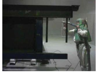
\*Production and consumption rates may vary based on nozzle size, pressure at the nozzle, standoff distance, abrasive metering, equipment quality, surface type, coating type and thickness. The blasting rates are achieved by setting the nozzle pressure to operate within the range of 95 psi – 100 psi. GMA will work with you to produce optimum performance on blasting jobs, reducing time and cost, and producing the best surface result for any coating.
